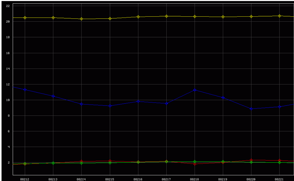
Fig 2. Speeds of the cart, true wind, and ratio thereof for the 10 second measurement period.
